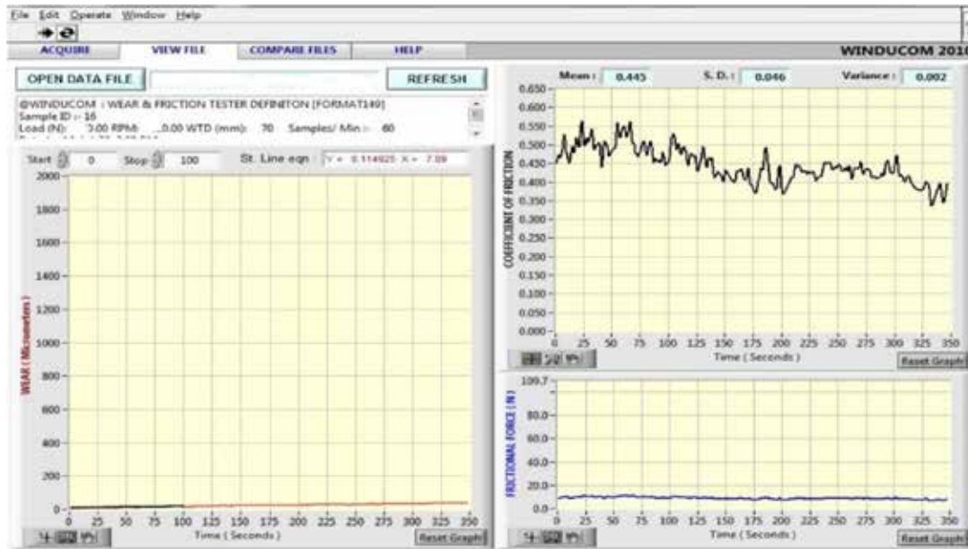
Fig.3. (a)Wear graph at Load = 10N, velocity =0.5m/s and distance = 500
