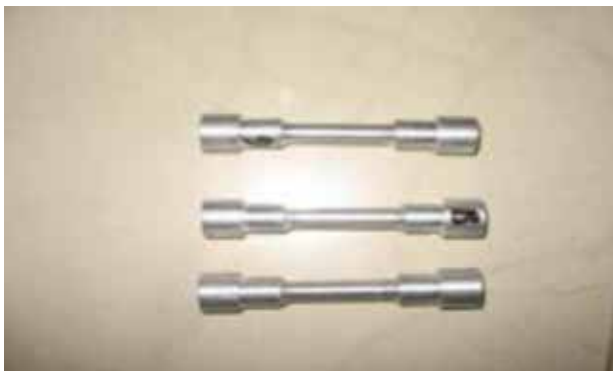
Fig-2: Tensile test specimens
