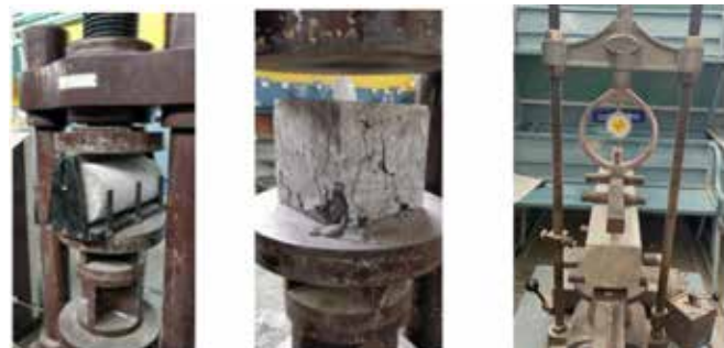
Fig. 3. Compression test, split tensile test, and flexural test
