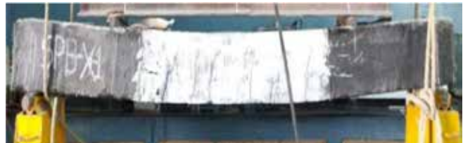
Figure 16 X1 failure mode
