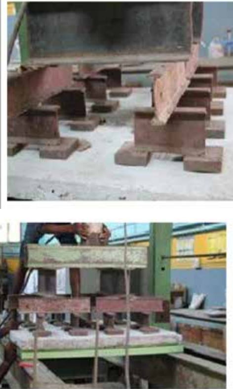
Fig. 5. Setup of slab with UDL arrangement
