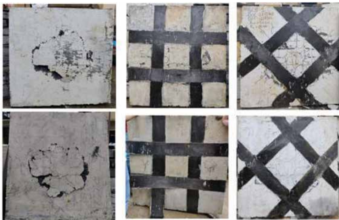
Fig. 4. Crack patterns in slabs. a) Control specimen, b) specimen with orthogonal wrapping pattern, c) specimens with skew wrapping pattern
