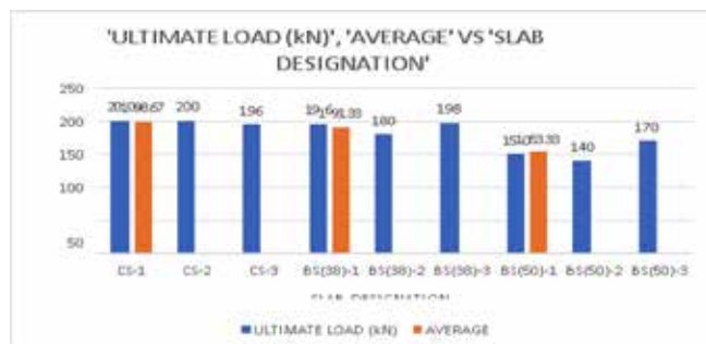
Comparison of ultimate load vs slab designation
