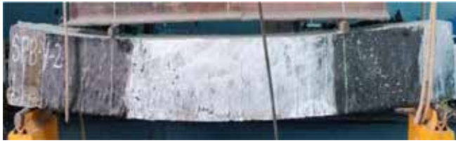
Figure 13 Crack pattern in SPB Y2
