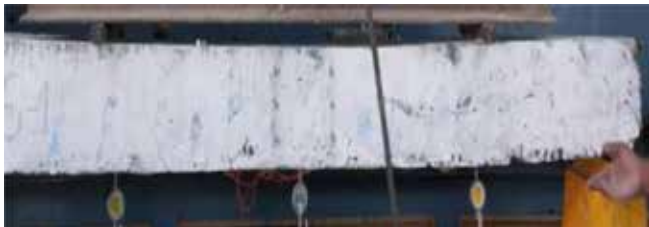
Figure 15 Control beam failure mode
